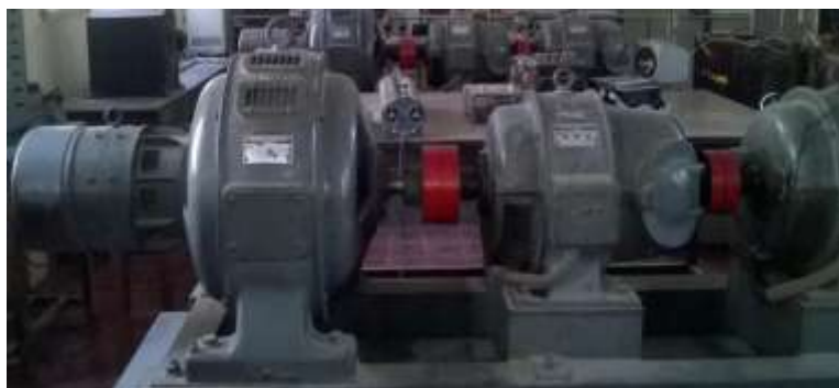
Fig. 1: Two alternators which we have synchronized
