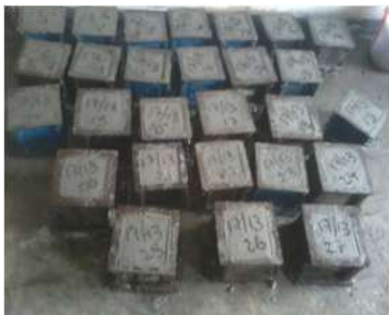
Fig.5 cubes after casting
