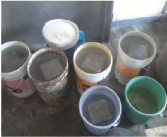
Fig.8 Cubes cured in sea water
