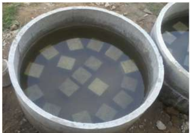
Fig.6 Cubes cured in normal water
