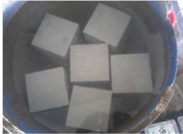
Fig.7 cubes cured in 1% H 2 SO 4 solution
