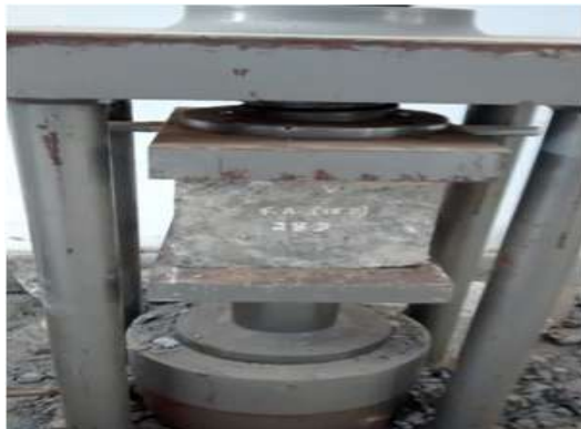
Fig.3 Cube specimen under compression
