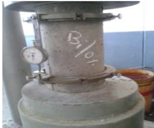
Fig.4 Cylinder under C.T.M during testing
