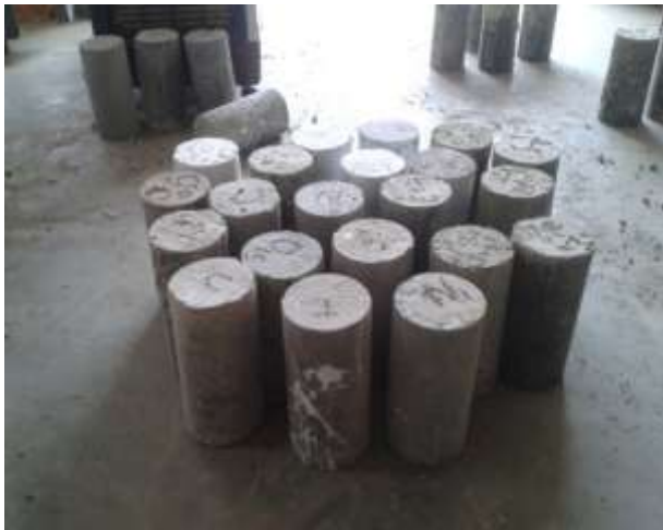
Fig.3 Cylindrical Specimens before testing
