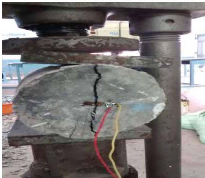
Fig.5 Cylinder during Split-tensile Test
