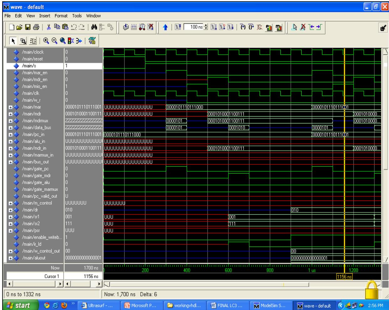
Figure 12: Detailed functional simulation diagram of Dual core LC3 processor executing AND.
