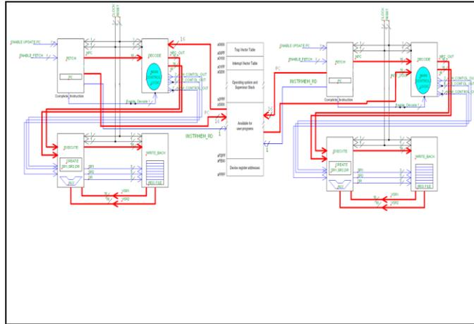
Figure 10: Dual-core SMP organization using LC3.
