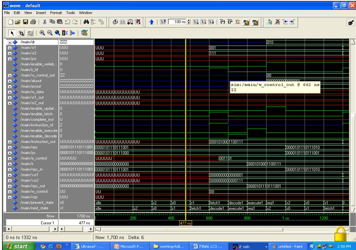
**Figure 13: Detailed functional simulation diagram of Dual core LC3 processor executing AND.**
