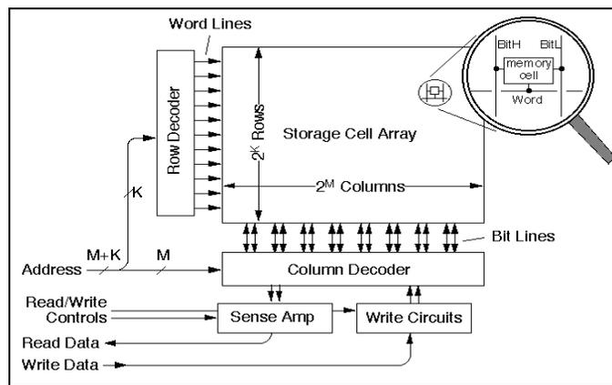
Figure 11: Typical memory architecture.
