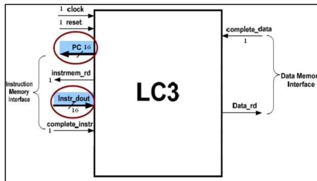
Figure 3: Entity diagram of the LC3 processor.
