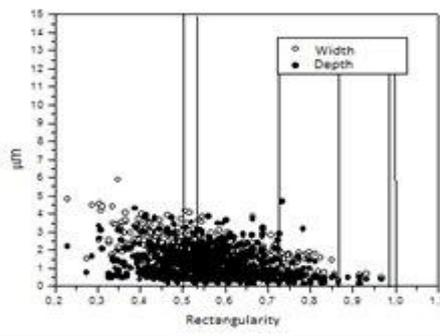
Fig. 8(a) - Size of pits formed on surface of stainless steel 304 in as-received state, after being subjected to corrosion tests via salt spray for 48 h.
