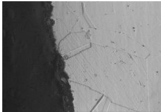
Fig. 5(b) - Occurrence of pitting corrosion in stainless steels 304, treated at 620 °C - 24 hours and air cooling.
