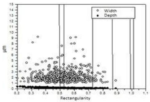
Fig. 8(b) - Size of pits formed on surface of stainless steel 304 in as-received state, after being subjected to corrosion tests via salt spray for 312 h.
