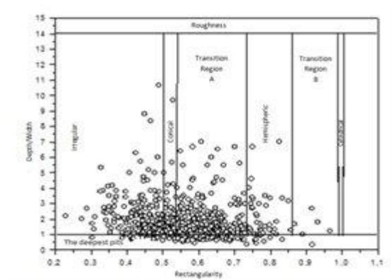
Fig. 6(a) - Classification of pits formed on surface of stainless steel 304 as received, subjected to corrosion tests via salt spray for 48 hours.
