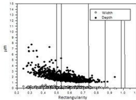
Fig. 9(b) - Size of pits formed on surface of stainless steel 304, treated at 620 °C for 24 hours and air cooling also subjected to corrosion testing via salt spray for 312 h.
