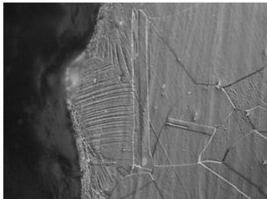
**Fig. 4(a) - The occurrence of pitting corrosion on stainless steel 304 in the state as received.**
