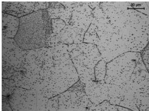
**Fig. 3 - Micrograph of 304 stainless steel treated at 620 °C - 24 hours, air cooling, etched.**
