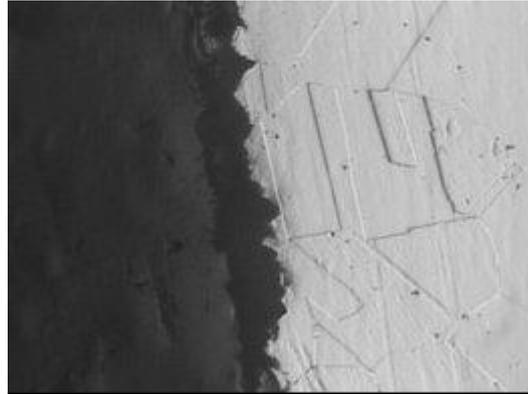
Fig. 5(a) - Occurrence of pitting corrosion in stainless steels 304, treated at 620 °C - 24 hours and air cooling.
