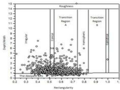
Fig. 7(b) - Classification of pits formed on surface of stainless steel 304 treated at 620 °C for 24 hours and air cooling and subjected to corrosion testing via salt spray for 312 hours.
