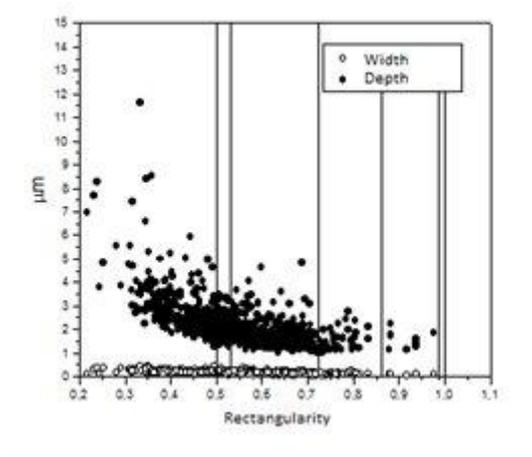
Fig. 9(a) - Size of pits formed on surface of stainless steel 304, treated at 620 °C for 24 hours and air cooling also subjected to corrosion testing via salt fog spray for 48 h.
