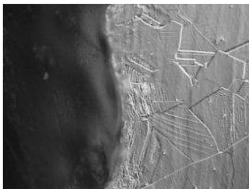
**Fig. 4(b) - Occurrence of pitting corrosion on stainless steel 304 in the state as received.**
