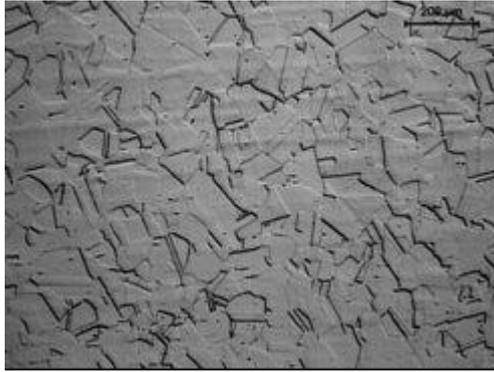
**Fig. 2 - Micrograph of AISI 304 stainless steel as received, etched.**
