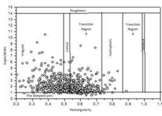
Fig. 6(b) - Classification of pits formed on surface of stainless steel 304 as received, subjected to corrosion tests via salt spray for 312 hours.
