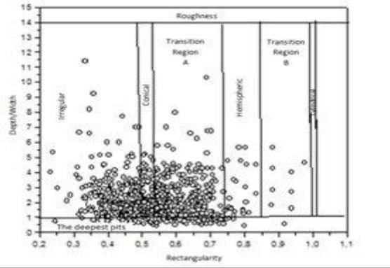
Fig. 7(a) - Classification of pits formed on surface of stainless steel 304 treated at 620 °C for 24 hours and air cooling and subjected to corrosion testing via salt spray for 48 hours.
