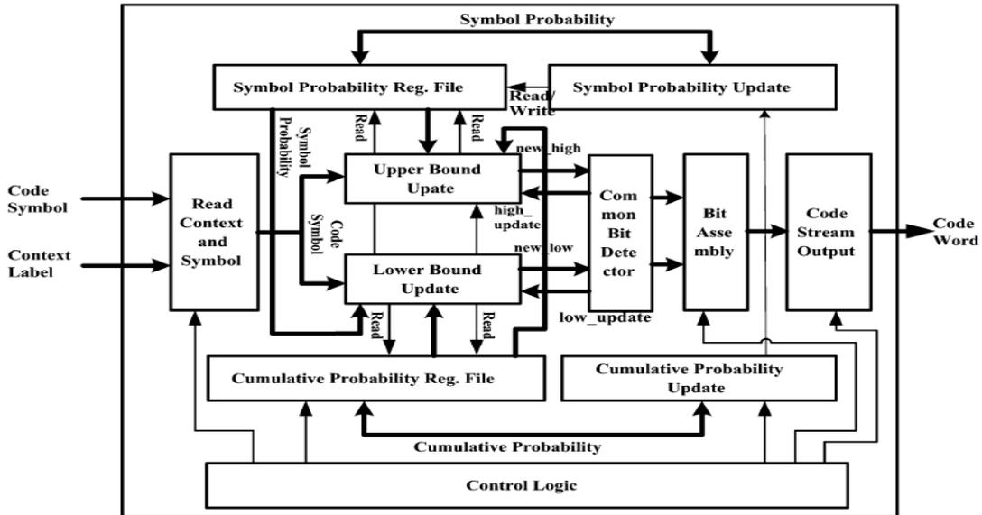
Fig. 4 Internal structure of arithmetic coder.
