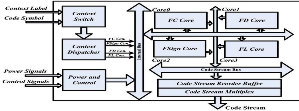
Fig. 3 Arithmetic coder's core structure.
