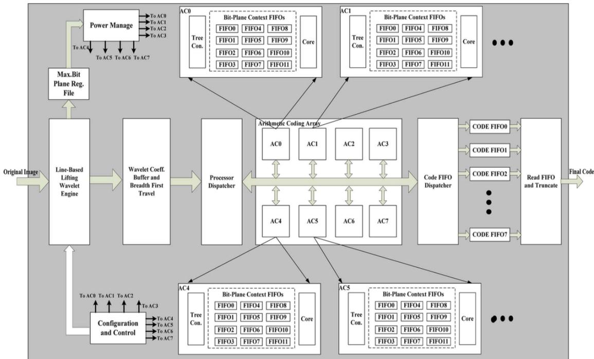
Fig. 2 Architecture of SPIHT encoding
