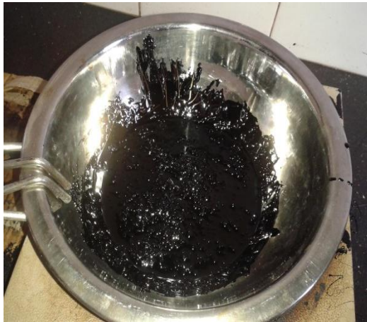
Fig.2. PP fibres mixed with bitumen
