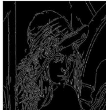
Figure 1. Cover Image using canny
