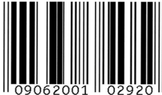
The bar code reader can manage different bar code standards even without having the knowledge of the standard code. The disadvantage with bar coding is that the bar scanner is unable to read if the bar code is concealed with grease or dirt.
