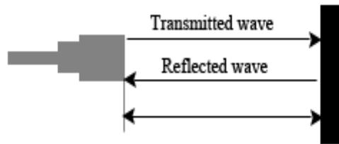
Since ultrasonic sensors rely on sound rather than light for detection, it is widely used to measure water-levels, medical scanning procedures and in the automobile industry. Ultrasonic waves can detect transparent objects such as transparent films, glass bottles, plastic bottles, and plate glass, using its Reflective Sensors.
