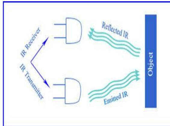
When IR receiver is subjected to infrared light, a voltage difference is produced across the leads. Less voltage which is produced can be hardly detected and hence operational amplifiers ([Op-amps](#)) are used to detect the low voltages accurately.
