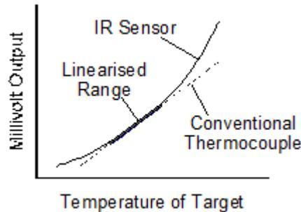
MES Infra-red sensors obtain all their power from the energy radiated from the target so, in order to minimize errors, the leakage current drawn by the attached measuring device must not exceed 10nA.
