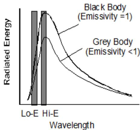
All real objects have a lower emissivity than an ideal black body and therefore radiate less energy. Shiny metal surfaces have a low emissivity, in the region of 0.05 to 0.2, whilst non-metals, organic materials and coated metals typically have high emissivity, in the range of 0.8 to 0.95. McLaren Electronics offers Infra-red sensors suitable for the high emissivity range of 0.8 to 0.98.
