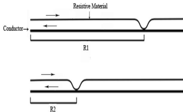
A touch sensor is made of: Fully conductive substance such as copper Insulated spacing material such as foam or plastic partially conductive material
