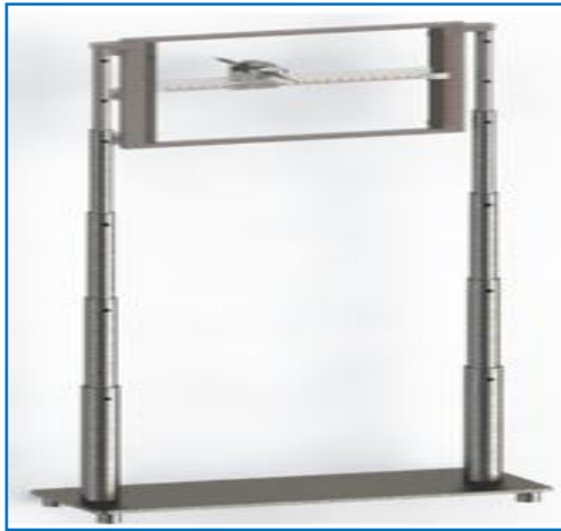
Fig. 2: Extensible support frame.
