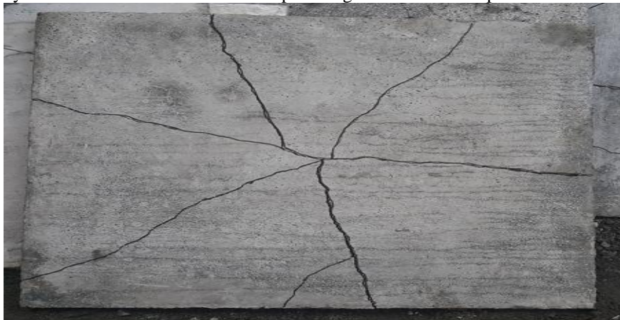
Fig.5: Crack pattern in slab with single layer of wire mesh
