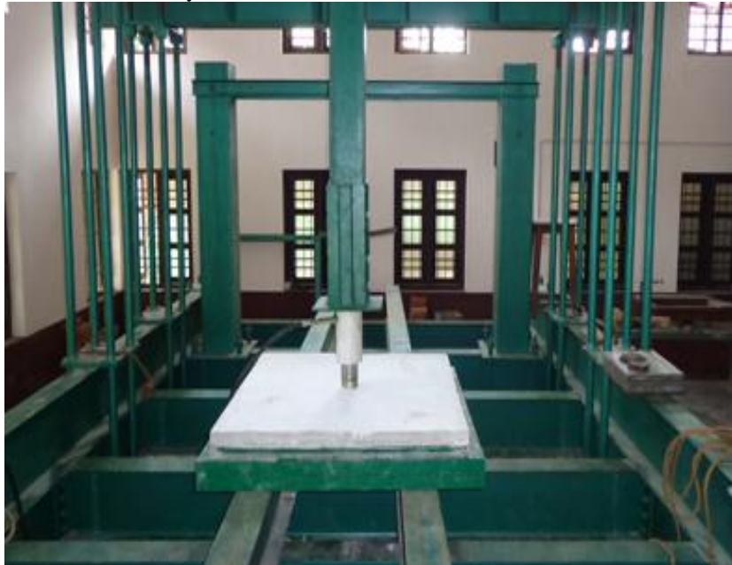
Fig.3: Slab placed on loading frame for testing
