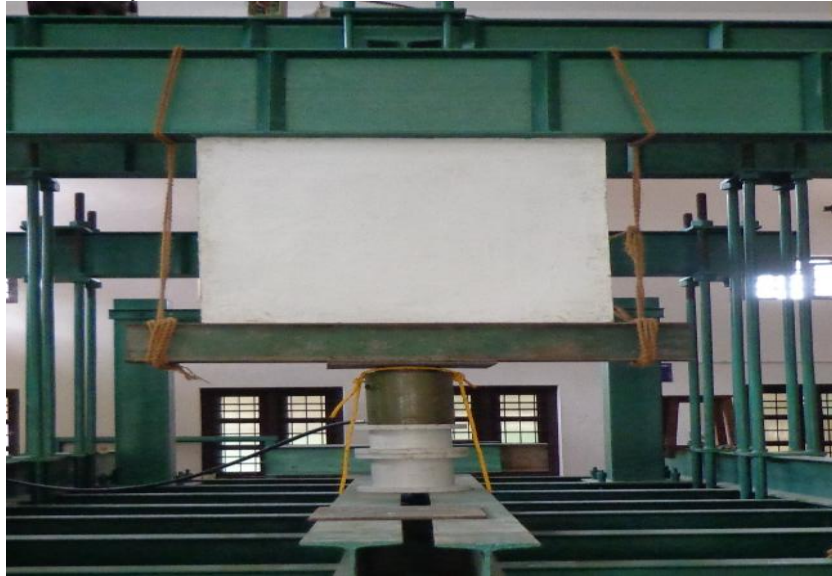
Fig.3: Wall panel placed on loading frame for testing
