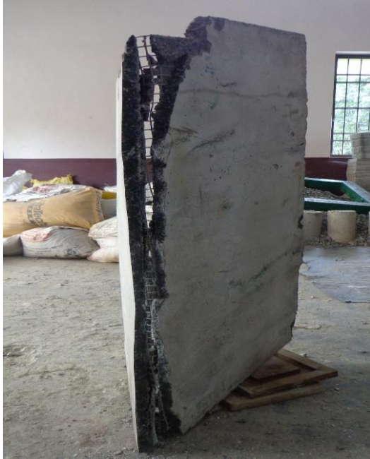
Fig.5: Crack pattern in slab with single layer of wire mesh
