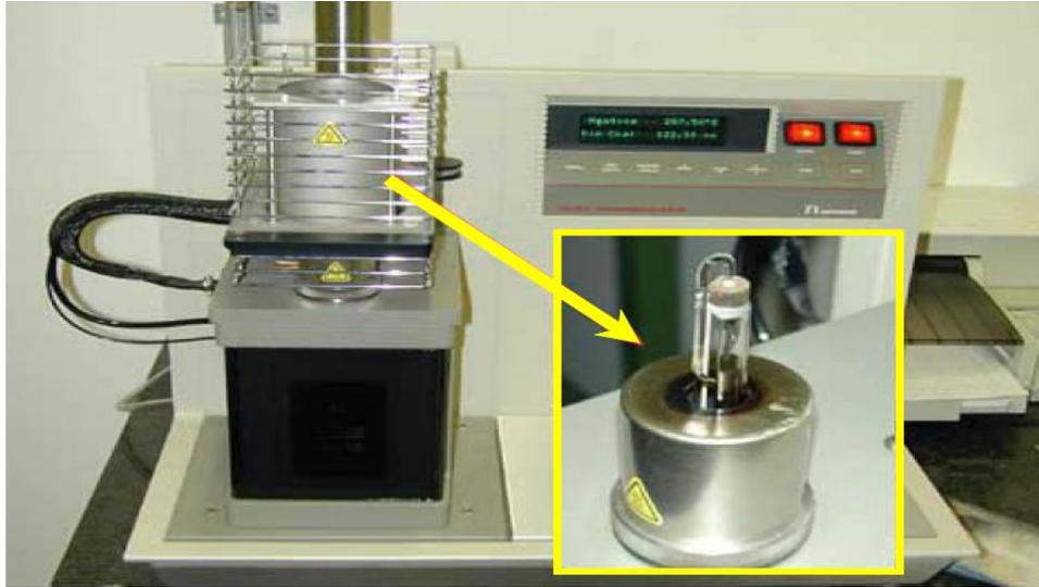
**Figure 4: TMA equipment to determine temperature profiles.**
