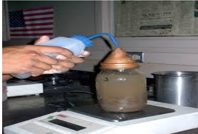
Fig.1 Pycnometer with quarry dust and water
