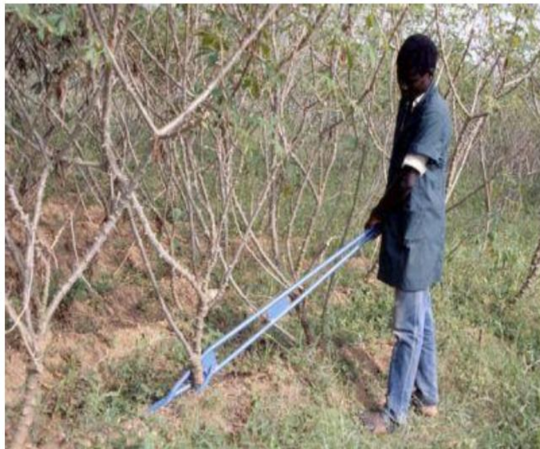
Figure 3: The IITA cassava lifter in use
