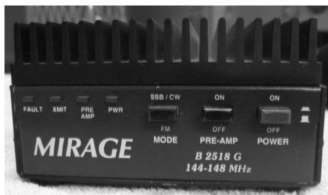
Fig. 3: A typical VHF Power Amplifier device
