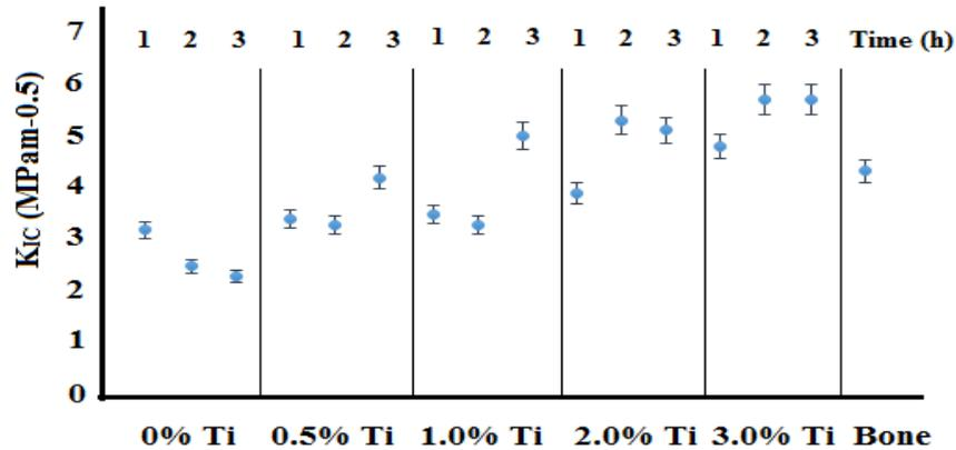
Fig. 2: Fracture toughness of composites Al<sub>2</sub>O<sub>3</sub>-X wt. % Ti, (X = 0.5, 1, 2 and 3), and fracture toughness of human compact bone
