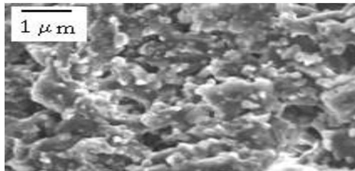
**Fig. 7:** Fracture surface in an Al<sub>2</sub>O<sub>3</sub>/Ti reinforced composite
