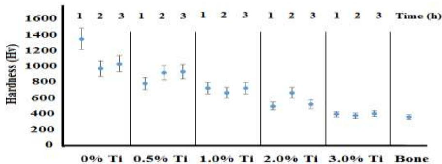
Fig. 3: Hardness of composites Al<sub>2</sub>O<sub>3</sub>-X wt. % Ti, (X = 0.5, 1, 2 and 3), and hardness of human compact bone
