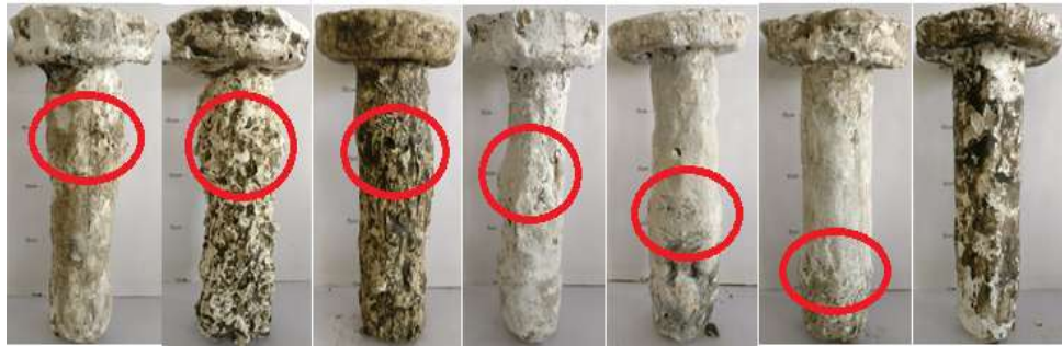
Fig. 4: Bulging of Stone column (Plain stone column with Stone aggregates, Slag, Slag+ Sand, Reinforced stone columns with encasement lengths of D, 2D, 3D, 4D respectively)
