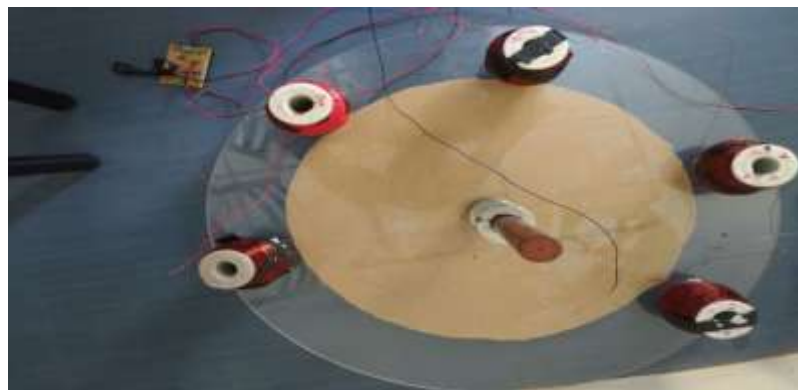
Fig.2 Top view of copper coils are placed in circular fashion with central axis wood rod
