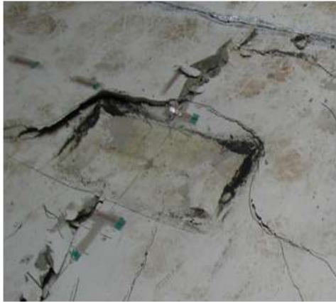
(a) Punching shear pattern around the loading plate (b) Method for determining the critical section
