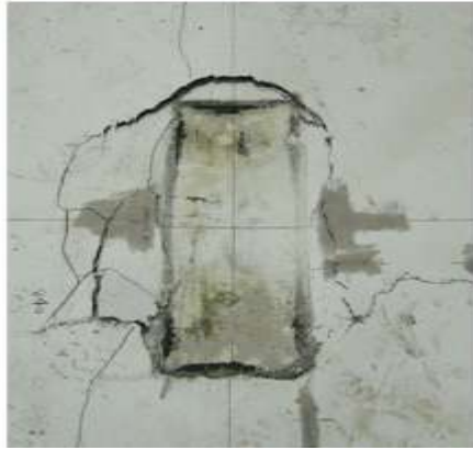
(a) Punching shear pattern around the loading plate (b) Method for determining the critical section
