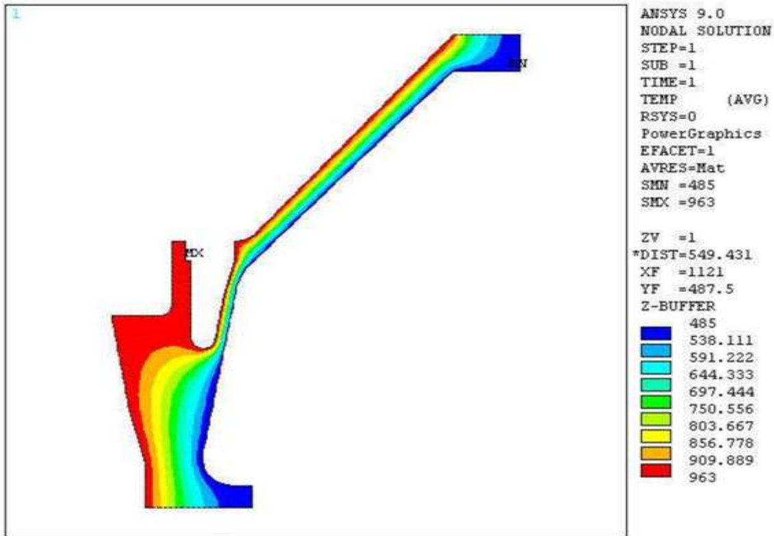
Fig. 17: Temperature Distribution Contours (Reduced Thickness of 15 mm)
