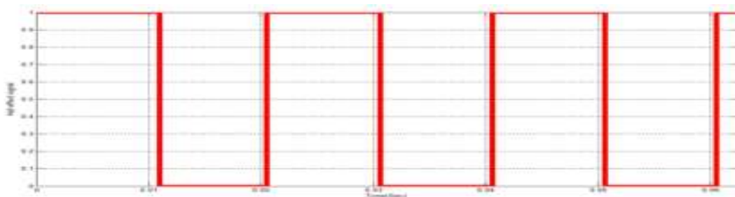
Fig.10: Hall Effect signal for phase A at no-load condition
