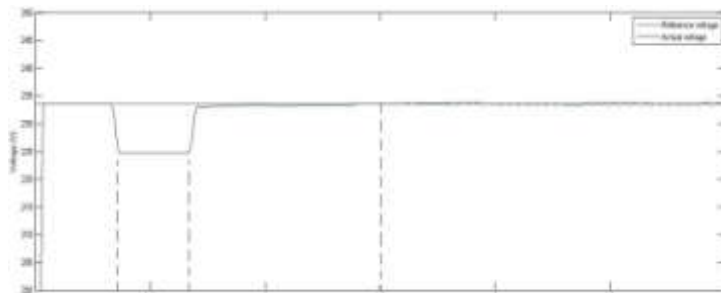
Fig.12. Voltage regulation with proper controller parameter
