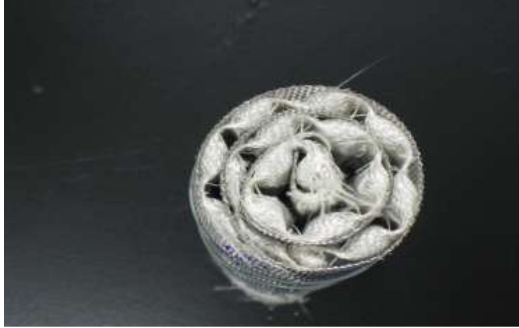
Figure 1. Bales Type Catalytic Packing
