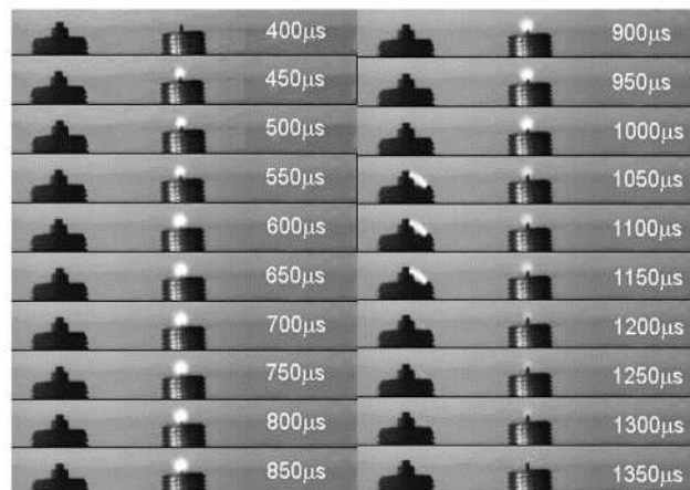
Figure 8. Ignition duration for typical spark ignited system (left plug) and the plasma igniter system (right plug) [29]
