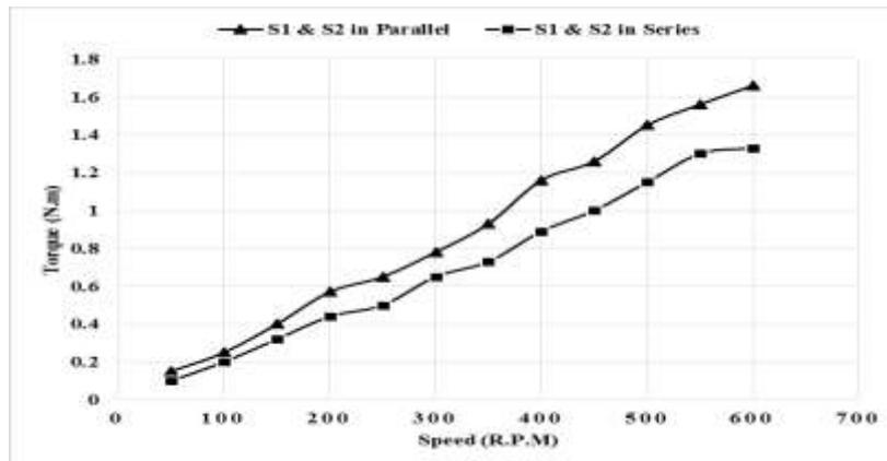
**Fig.9:** The electromagnetic torque at load  $50\Omega$
