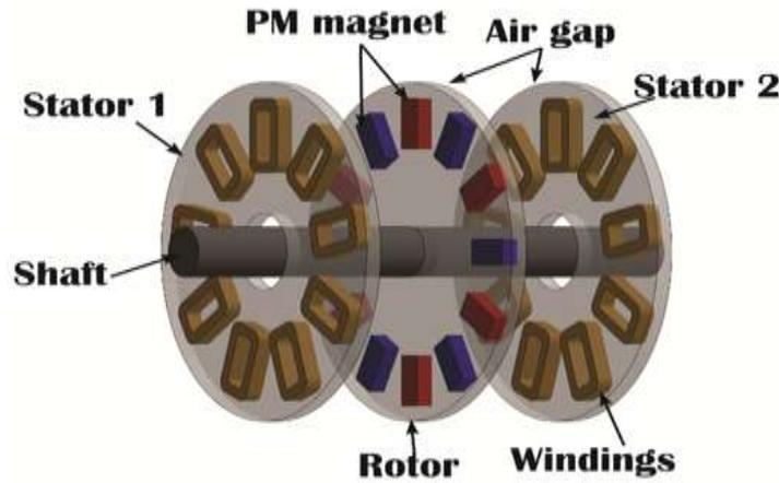
**Fig.1:** Construction of AFPM Generator (double stator – single rotor)
