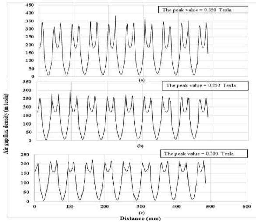
**Fig.3:** The peak value of flux density in the air gap with deferent sizes :,(a) Air gap (2 mm), (b) Air gap (4 mm), (c) Air gap (6 mm),
