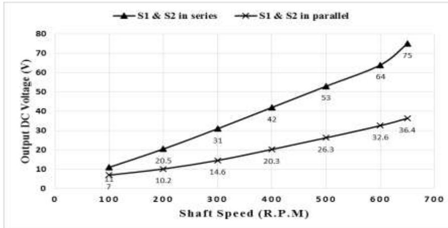
**Fig.5:** The output voltage of two stators ( $S_1$ & $S_2$ ) at no load connected in parallel and in series
