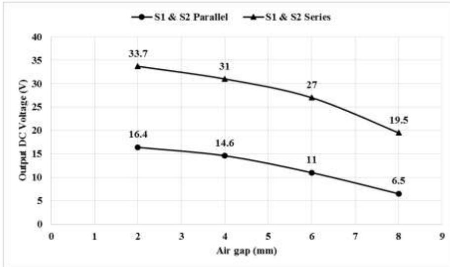
**Fig.8:** The air gap effect on the output voltage of the generator at fixed speed (300 r.p.m)
