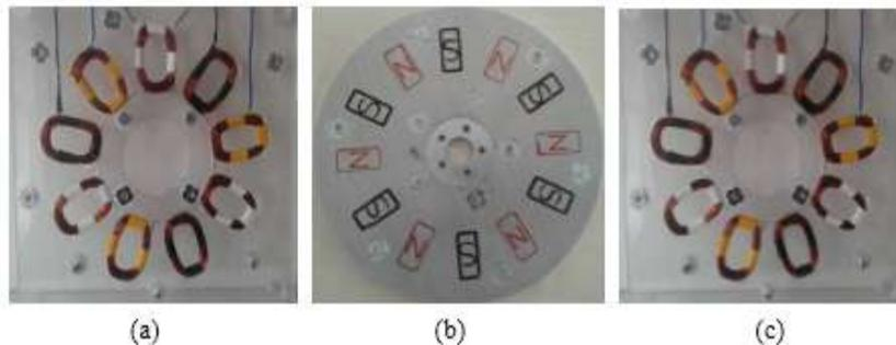
**Fig.2:** (a) The stator (I), (b) The stator (II) is manufactured by using a non-ferromagnetic material with the coils (Plexiglas), and (c) The rotor is a circular non ferromagnetic material(aluminium) with permanent magnets
