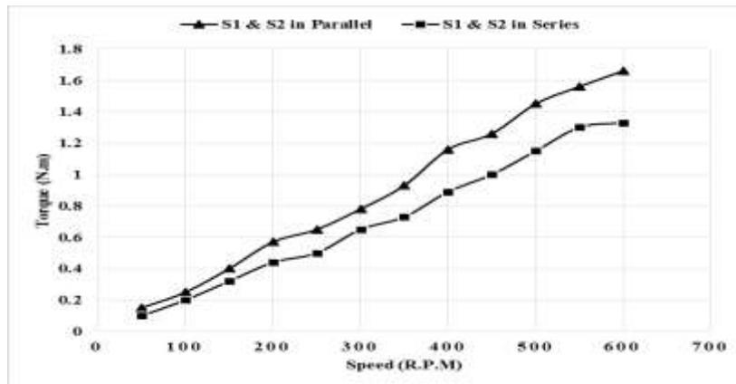
**Fig.9:** The electromagnetic torque at load 50Ω
