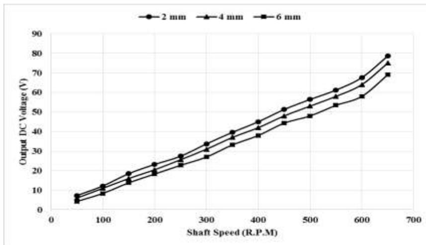
**Fig.6:** The air gap effect on the output voltage of the generator when ( $S_1$  &  $S_2$  in series)
