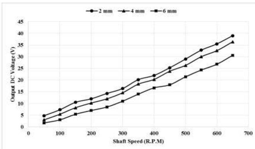
**Fig.7:** The air gap effect on the output voltage of the generator when ( $S_1$  &  $S_2$  in parallel)
