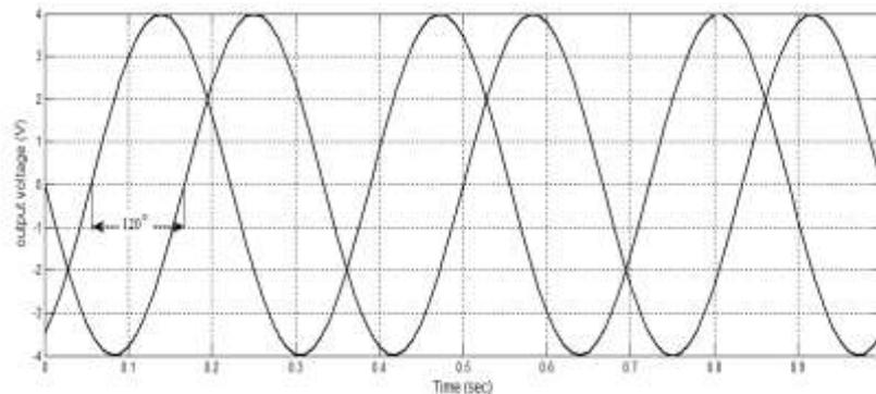
**Fig.4:** The output voltage at 100 rpm
