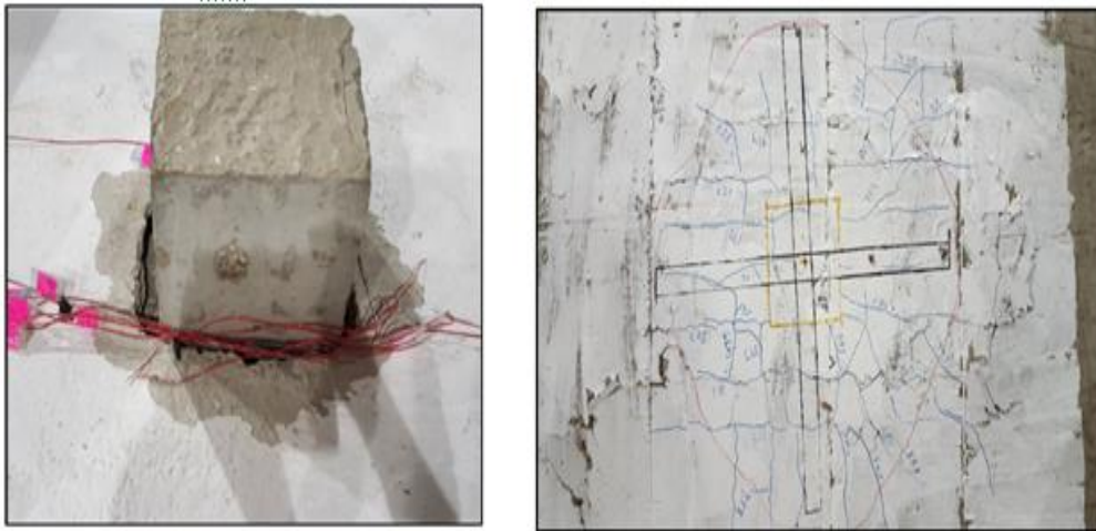
Figure (27): The crack pattern and mode of failure at the top and bottom of specimen "S-L2-2"
