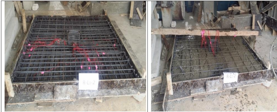
Figure (8): Specimen "R-L1-2" during preparing and placing of concrete in lab.
