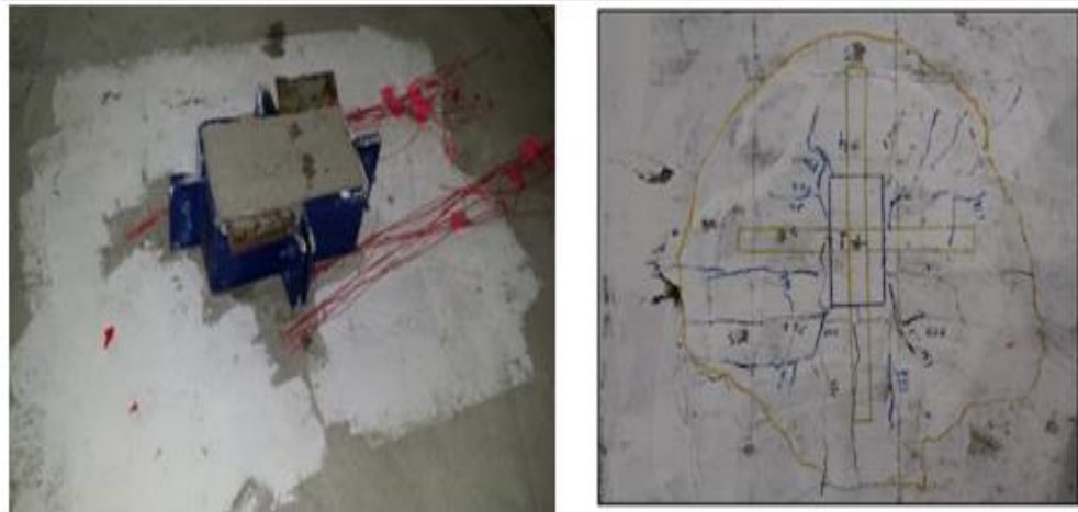
Figure (29): The crack pattern and mode of failure at the top and bottom of specimen "R-L1-2".
