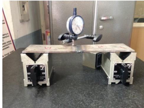
Fig 2.6 Angular distortion measurement
