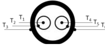
Fi.13: Arrangement / assembling of the temperature sensors.
