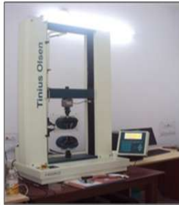
Fig. 9. UTM for tensile test (TINIUS OLSEN, model no.- H50KS, 50 KN capacity)
