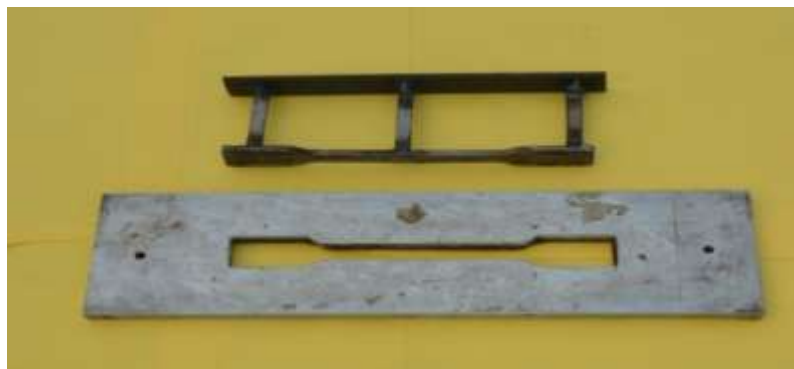
Fig.5. Metallic mould with ejector for standard specimen
