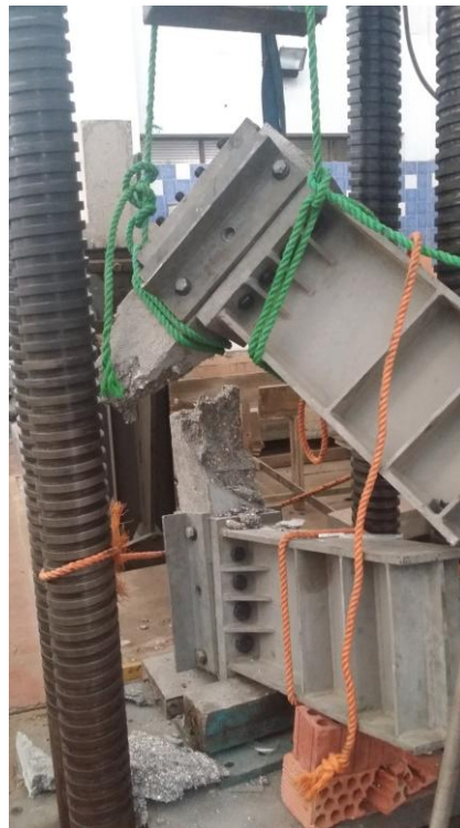
Fig.2: Crushing of the concrete of stress block parameter specimen.
