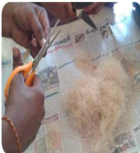
**Fig.3:** Cutting of fibers
