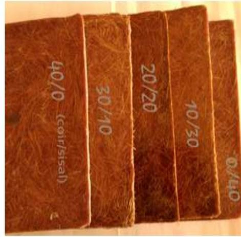
Fig.6: Final composite laminates
