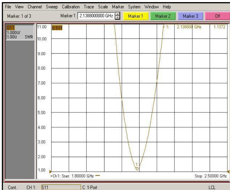
Fig.10. Measured Result of VSWR of Ant2.
