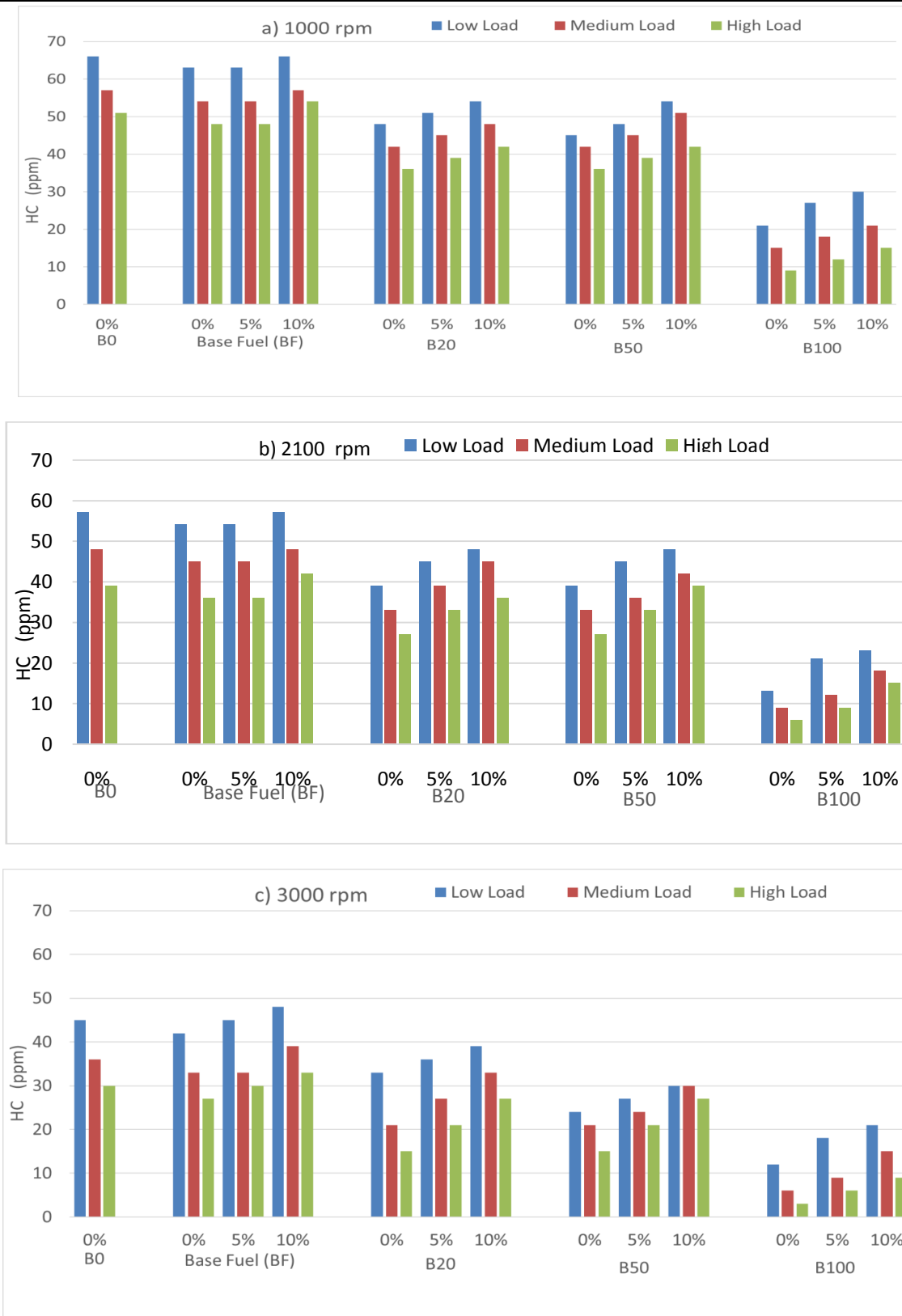
Figure 7: HC emissions of different fuel blends with 5% and 10% emulsification at a) 1000 rpm, b) 2100 rpm, and c) 3000 rpm
