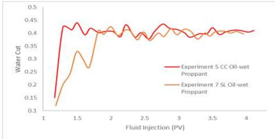
**Figure 10: Comparison SL 12/18 “oil-wet” proppant and CC 20/40 “oil-wet” proppant with oil injection followed by 40% water cut two-phase injection**
