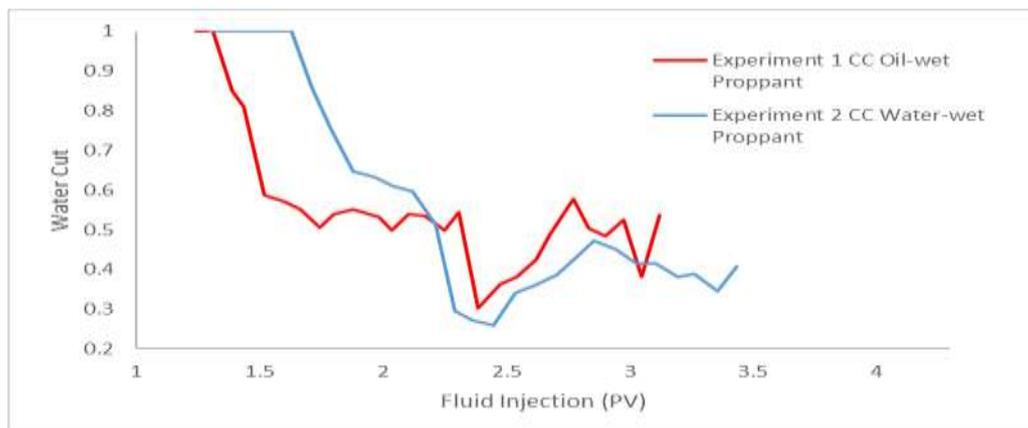
**Figure 7: Comparison of 20/40 “oil-wet” proppant and 20/40 “water-wet” proppant with 40% water cut two-phase injection**
