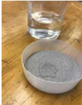
(a) Water was absorbed by the proppant immediately, indicating water-wetting surface of the proppant.
