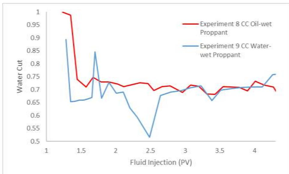
**Figure 11: Comparison of 20/40 water-wet proppant and 20/40 oil-wet proppant with Oil Injection Followed by 70% Water Cut Two-Phase Injection**
