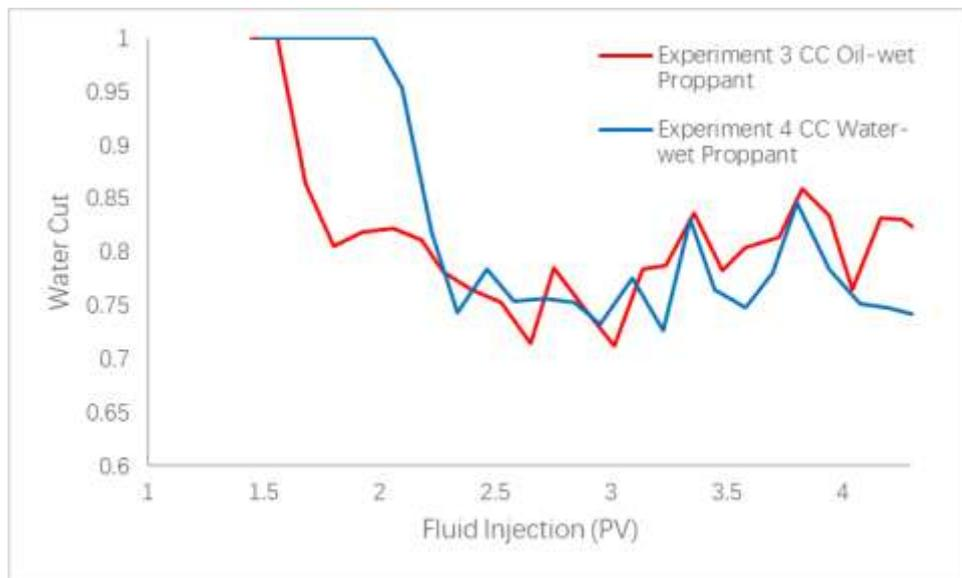
**Figure 8: Comparison of 20/40 “oil-wet” proppant and 20/40 water-wet proppant with 70% water cut two-phase injection**
