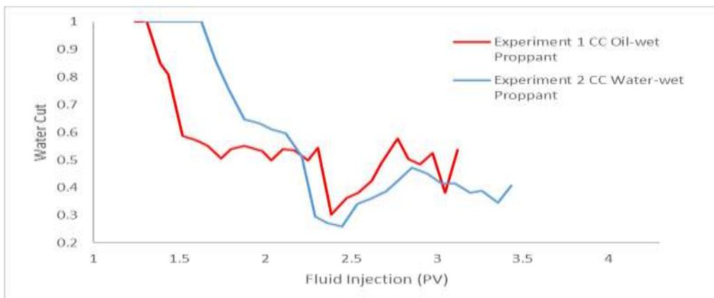
**Figure 7: Comparison of 20/40 “oil-wet” proppant and 20/40 “water-wet” proppant with 40% water cut two-phase injection**
