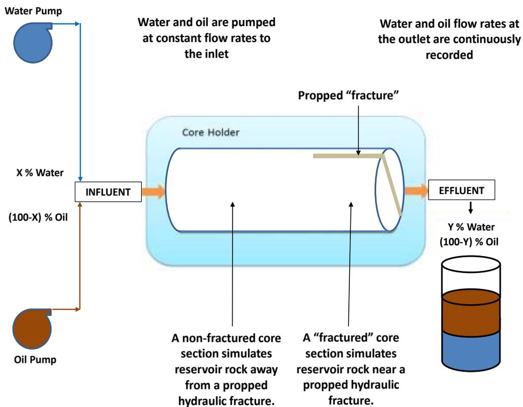
**Figure 3:** A flow diagram to show water-oil 2-phase injection
