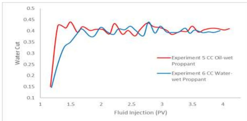
**Figure 9: Comparison of 20/40 oil-wet proppant and 20/40 water-wet proppant with oil injection followed by 40% water cut two-phase injection**
