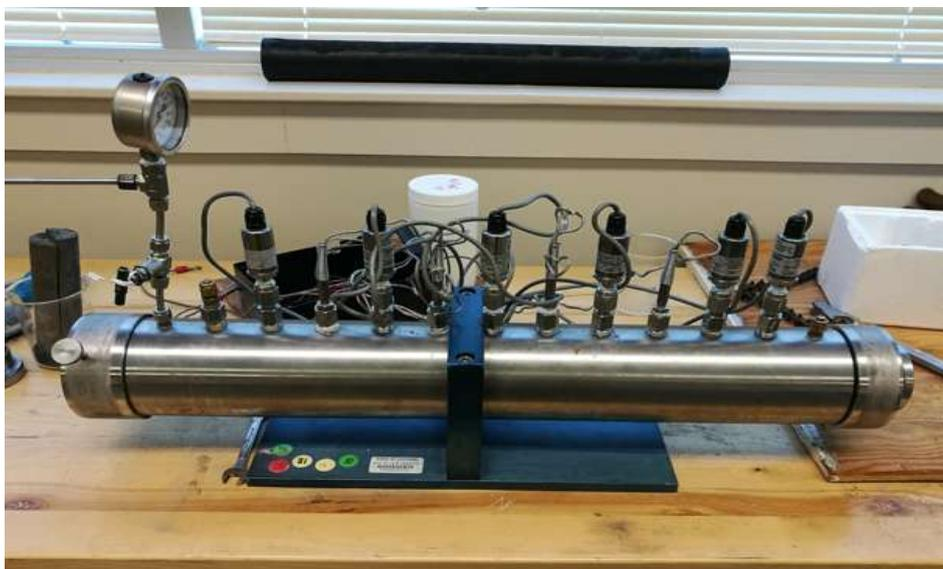
**Figure 1: Image of a 2-foot long core holder**
