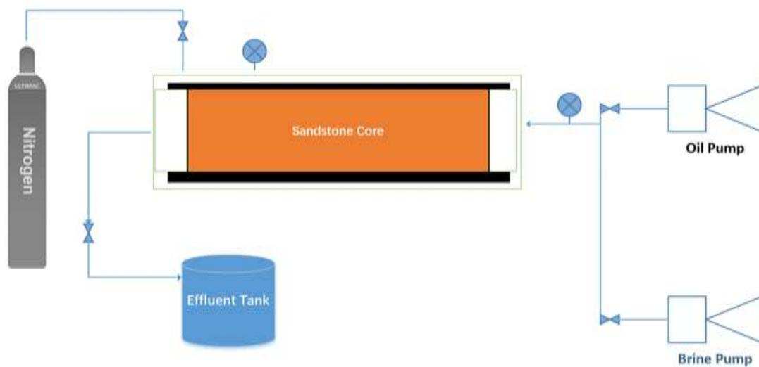
**Figure 2:** A schematic drawing the of core holder with surrounding connections
