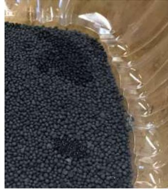
(b) Oil was absorbed by the proppant immediately, indicating oil-wetting surface of the proppant.
