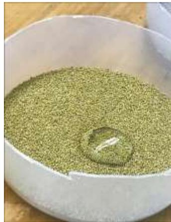
(a) Water was not absorbed by the proppant immediately, indicating non-water-wetting surface of the proppant.
