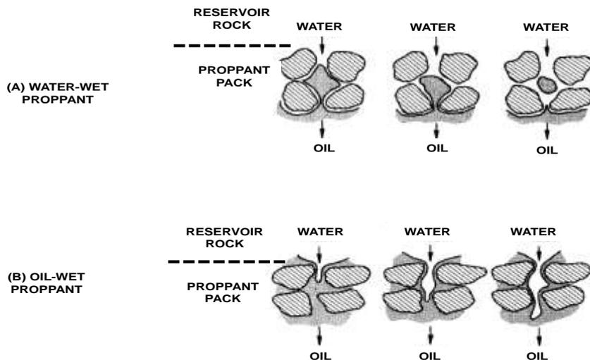
**Figure 12: Effect of proppant wettability on the fluid channel development at the fracture face (Modified from Raza et al. 1968)**
