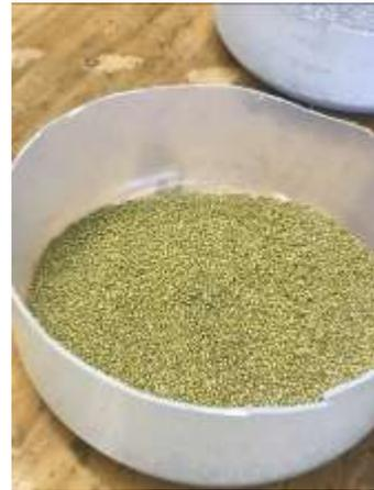
(b) Oil was absorbed by the proppant immediately, indicating oil-wetting surface of the proppant.
