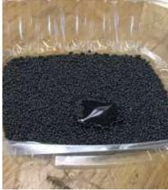
(a) Water was not absorbed by the proppant immediately, indicating non-water-wetting surface of the proppant.
