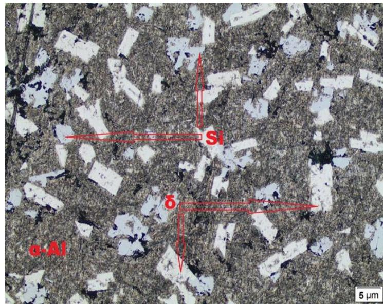
Figure 1: Optical microscopy micrograph of as cast AlCC3 (Al-Si-Fe-B) alloy.
