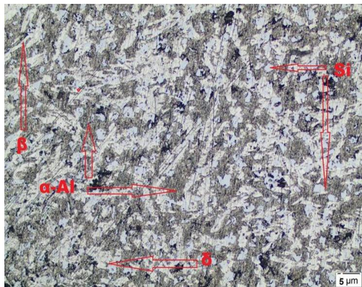
Figure 2: Optical microscopy micrograph of as cast AlCC4 (Al-Si-Fe-B-Ni) alloy.
