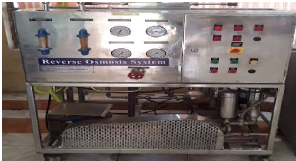
Figure - 5: Reverse Osmosis Setup
