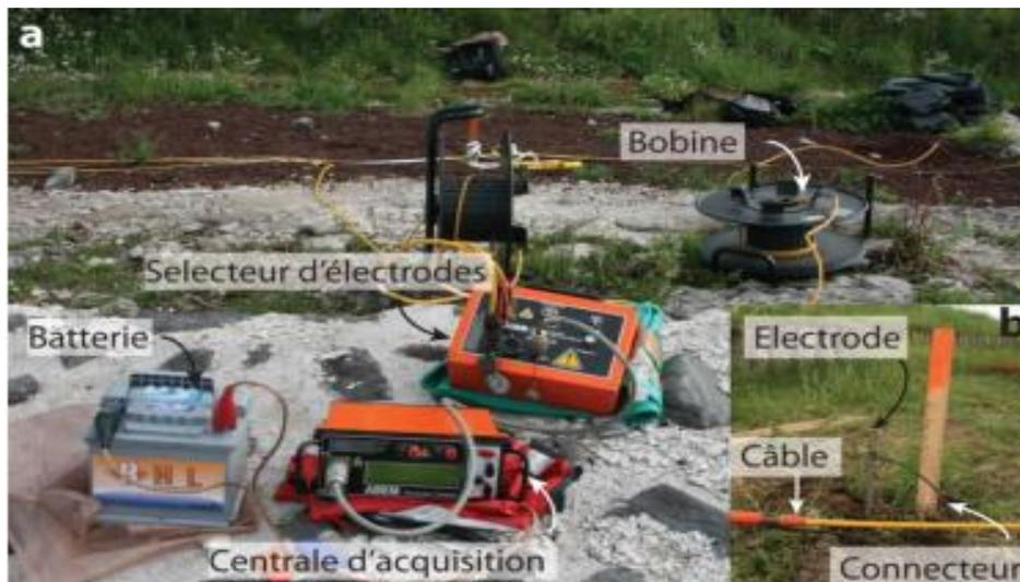
**Fig. 2: Experimental device ABEM SAS 4000; a) main equipment; b) electrode.**
