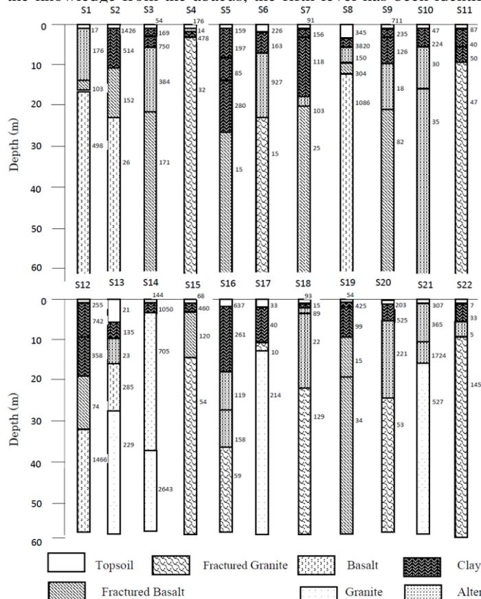
**Fig. 4: Geoelectric sections of the study area; the numbers represent resistivities in ohm-meter; The Si represent the different stations of the study area (i ranging from 1 to 22)**
