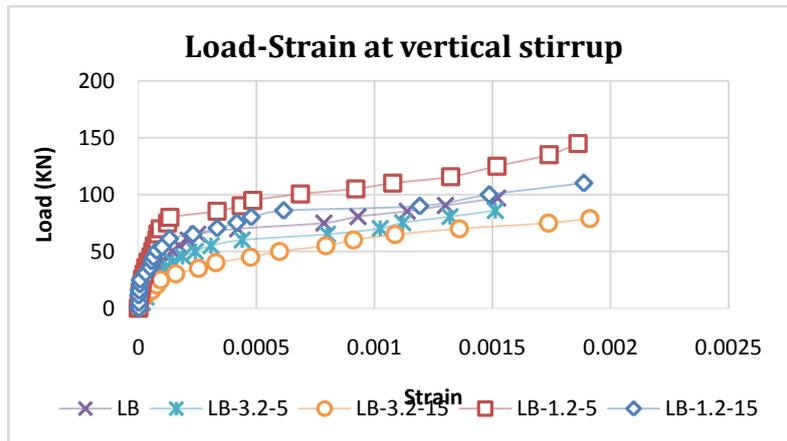
Fig.14b: Load-Strain at Vertical Stirrup Curve for G2 Specimens
