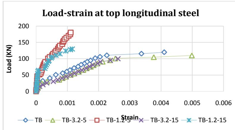
Fig.15a: Load-Strain at Upper Longitudinal Steel Curve for G1 Specimens
