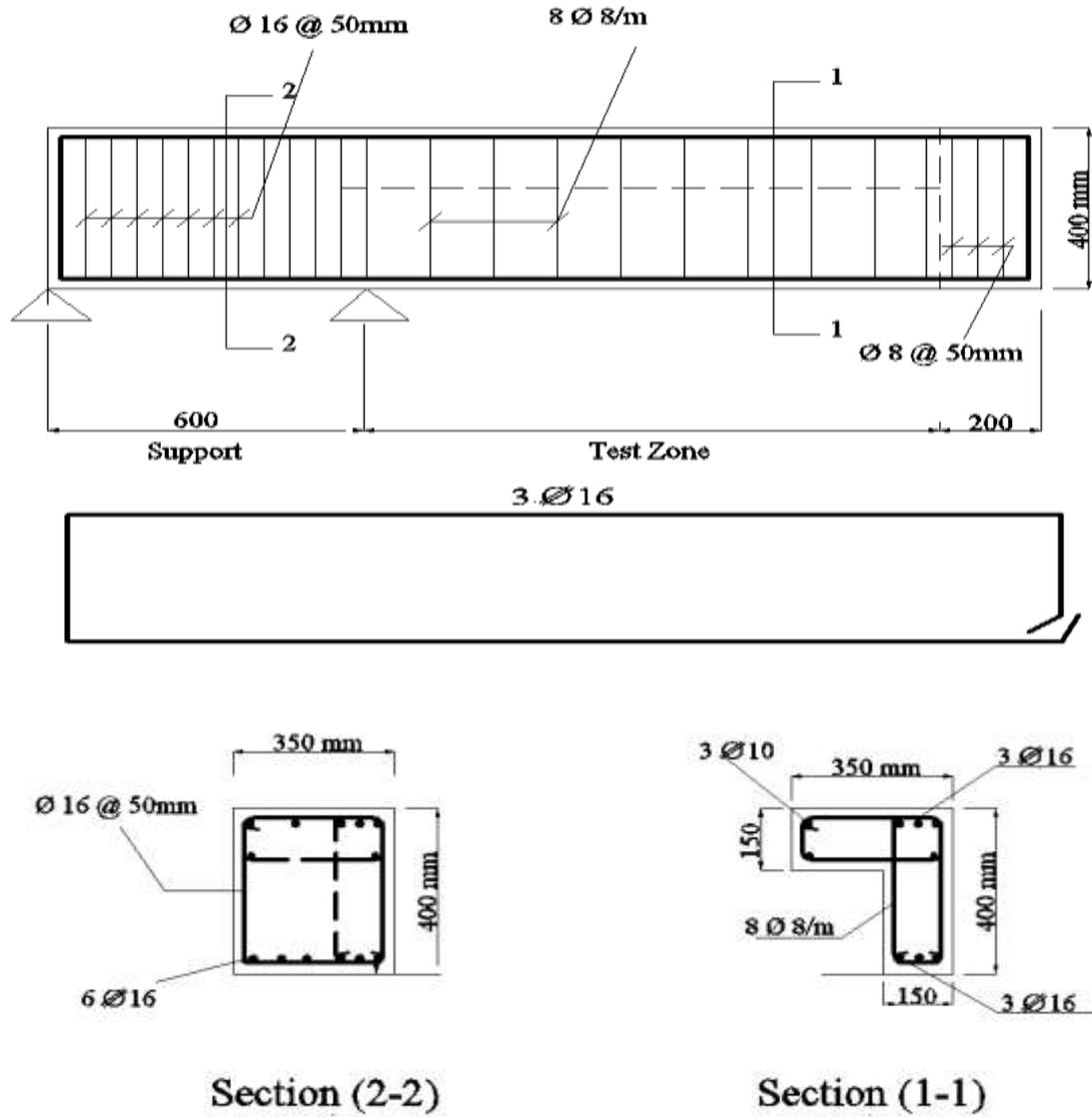
Fig.1b Typical dimensions and reinforcement of group G2
