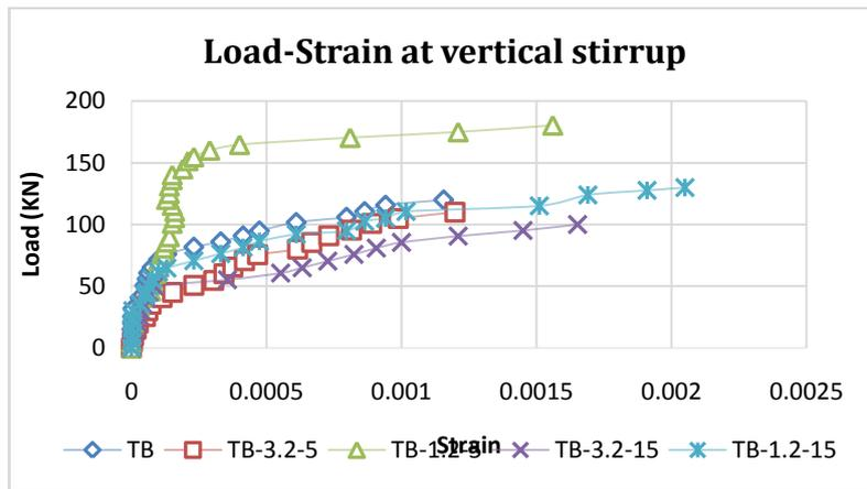
Fig.14a: Load-Strain at Vertical Stirrup Curve for G1 Specimens
