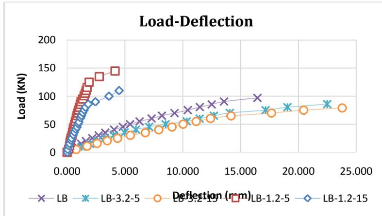
Fig.13b: Load-Deflection Curve for G2 Specimens
