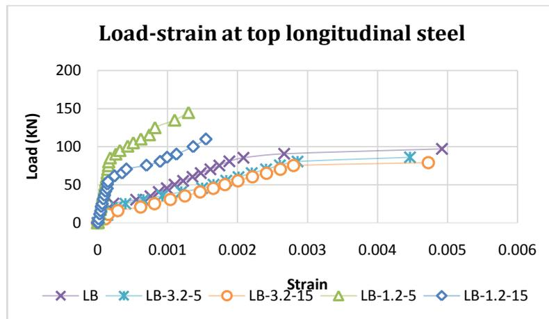
Fig.15b: Load-Strain at Upper Longitudinal Steel Curve for G2 Specimens
