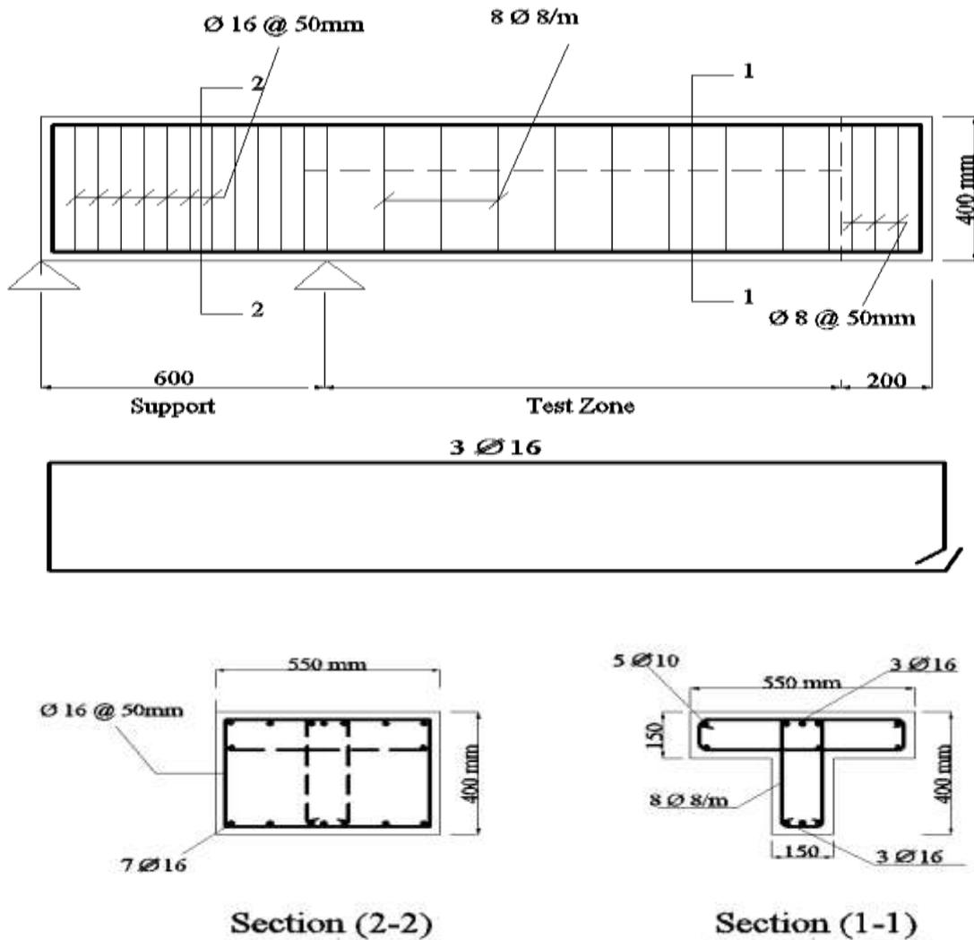
Fig.1a Typical dimensions and reinforcement of group G1
