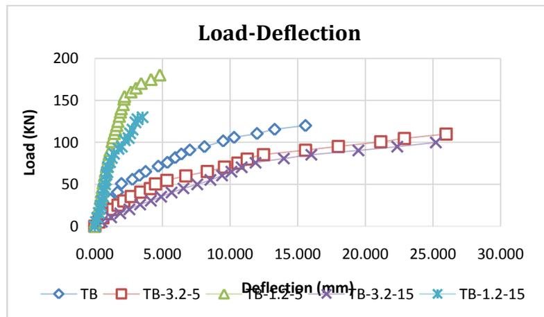
**Fig.13a:** Load-Deflection Curve for G1 Specimens
