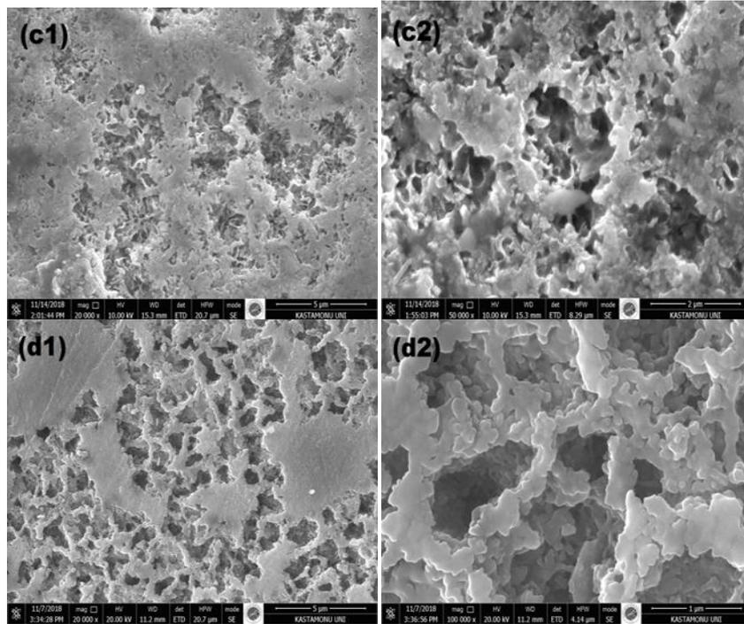
Figure 3: SEM images revealing the microstructure of AIMS3 (c1, c2) and AIMS2 (d1, d2).
