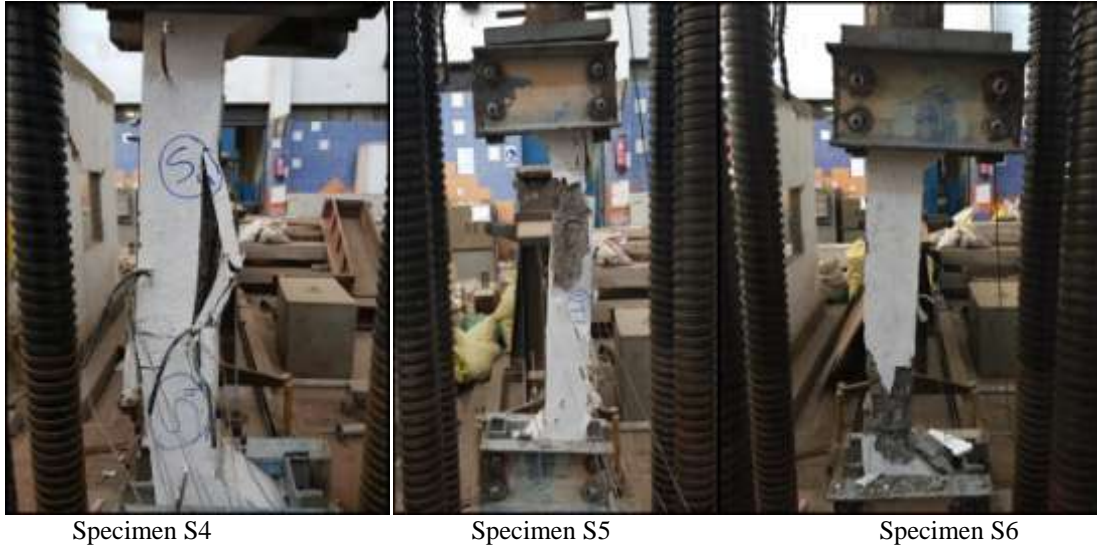
Figure 5: Failure patterns of the specimens
