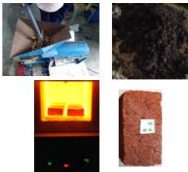
Figure 1: Raw materials (crushed mix of bamboo and ficus Alestica's leaves, clay) and shaped samples (fired brick in electric furnace left, fired brick right).
