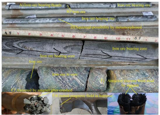
**Fig. 6.** Photograph showing the iron ore bearing core where clearly visible of A) iron bands, B) breaking surface ore concentration, C and F) crushing samples (by both hammer and drilling bit) attracted by magnet, E)
