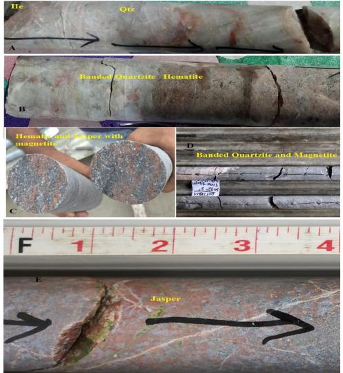
**Fig.8.** Photograph showing the A) alternation of quartzie and hematite, B) banded quartzie and hematite, C) hematite and jasper, D) banded quartzie and magnetite and E) core sample of jasper which are clear indication of BIF, Alihat, Hakimpur, Dinajpur, Bangladesh.
