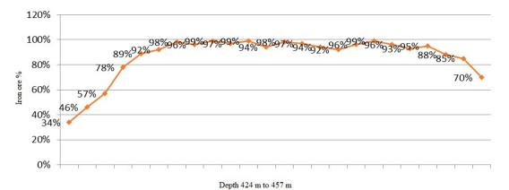
**Fig. 11.** Photograph showing the compositional variations of crushing test results or analysis in the field where shown high concentration of iron ore or magnetic minerals (34% - 99%) at Alihat, Hakimpur, Dinajpur, Bangladesh.
