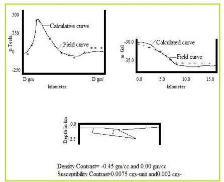
**Fig. 3.** Modeling of combined gravity and magnetic profile Cgm-Cgm and Dgm-Dgm Dinajpur and Rangpur Area (modified from Rahman et.al. 2000).
