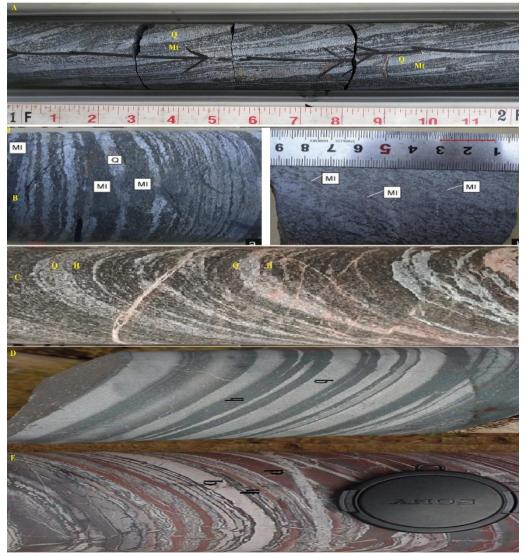
**Fig. 7.** Photograph showing the A) iron ore bearing core where alternation of quartz and magnetite like as B) those types of samples in China-BIF (Han, et.al, 2014). C) Sample of the study area where clearly visible
