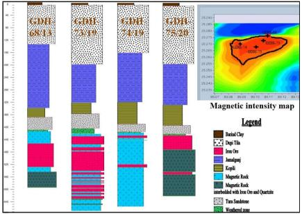
Fig. 5. Figure showing correlation of four drill hole logs and condition of iron ore layers and others lithological units, magnetic intensity map Alihat, Hakimpur, Dinajpur, Bangladesh.
