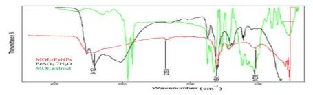
FTIR spectra of MOL-FeNPs, MOL extract, FeSO<sub>4</sub>.7H<sub>2</sub>O solution
