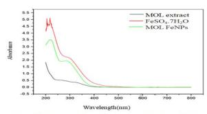
UV-visible absorption peak of MOL extract, MOL FeNPs and FeSO<sub>4</sub>.7H<sub>2</sub>O solution
