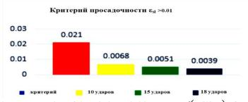
Figure 4. Diagram of the average value of the relative subsidence  $\varepsilon_{sl} = f(n, W_{opt})$  of compacted soil at different numbers of impacts
