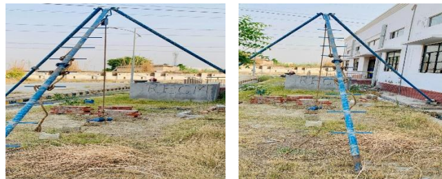
Figure 17: Experimental loading arrangement and masonry wall
