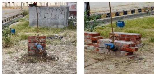
Figure 18: Distortion of masonry wall under impact load
