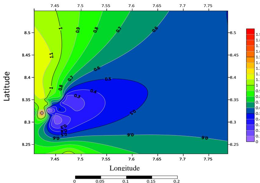
Figure 2: AVI vulnerability rating for groundwater in Makurdi
