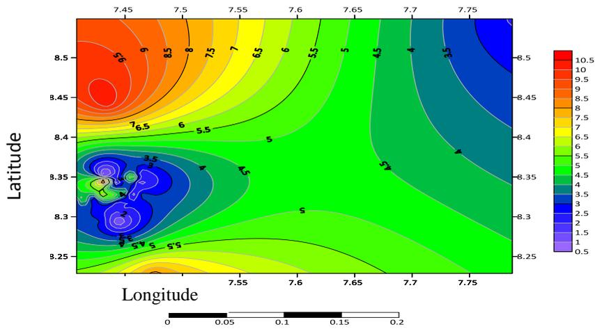
Figure 4: GLSI vulnerability rating for groundwater in Makurdi
