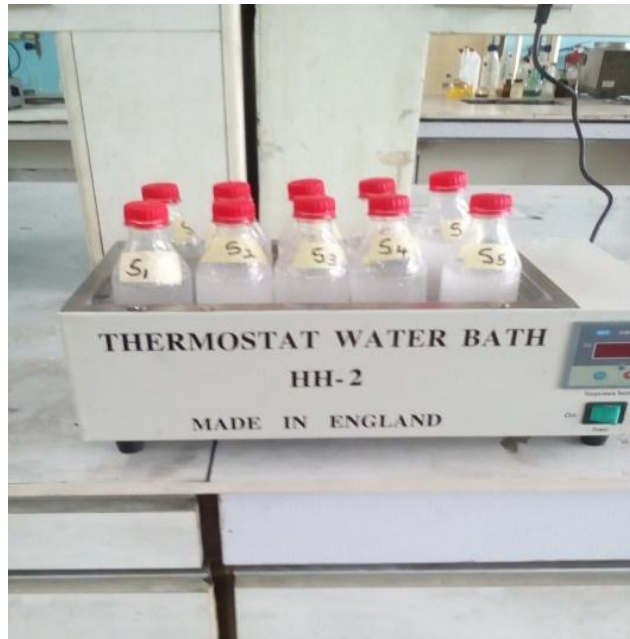
Figure 2: Experimental Set – up for Determining Cassava Wastewater (Substrate) Concentration
