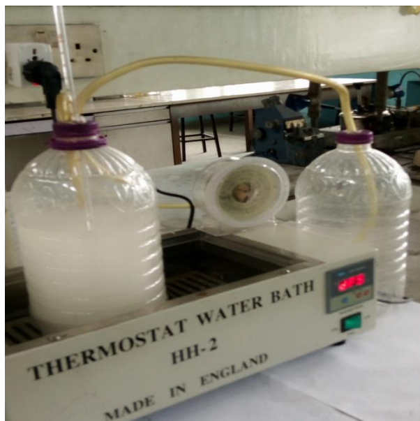
Figure 2: Experimental Set-up for Biogas Production
