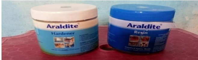
Hardener Resin 220 g of Hardener and 240 g of Resin Mixture at one Ratio
