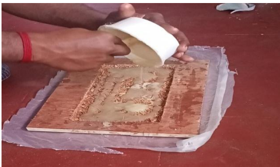
Resin pouring to the mould cavity
